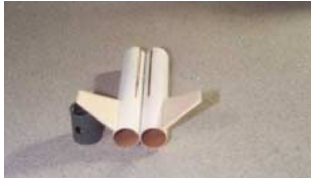
Figure 3-6 – Stabilizers Installed and Drying
